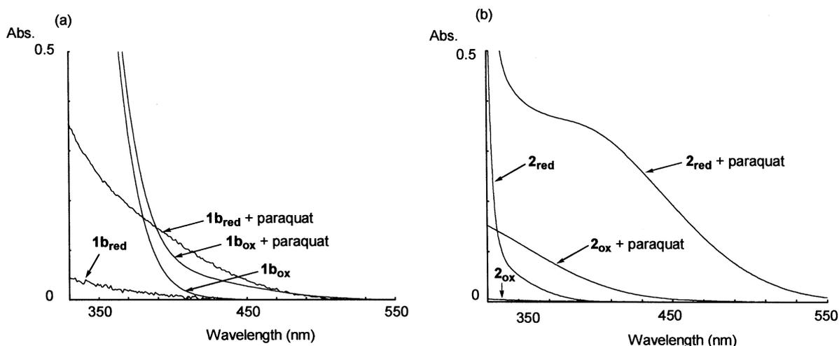
**Figure 2.** UV-vis spectroscopic changes of (a) **1** and (b) **2** by the addition of 1.0 equiv. of paraquat ([host]=2.0 mM, CDCl<sub>3</sub>:CD<sub>3</sub>CN=1:1).
